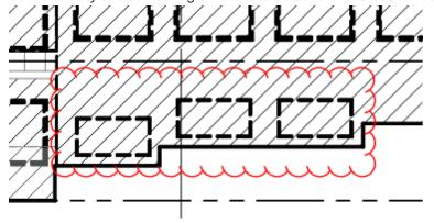
A) Dashed line currently shown in elevation drawings indicates existing windows to be removed.
