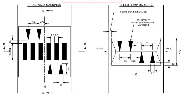
\* $\underline{\mathsf{NOTE}}$ : For STAMPED PAVER crosswalks, EDGES to be marked by parallel lines.
