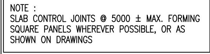
CONTROL JOINT FOR SLAB ON GRADE (NON-WATER RETAINING STRUCTURES)
